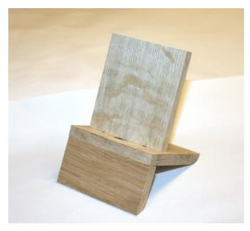
Put some glue onto the top of the foot and press foot and base firmly together. (With a clamp). Take special care that the sides are at the justified with the base. A proven method is to do this on the corner of a table and to put the clamps from the site.
